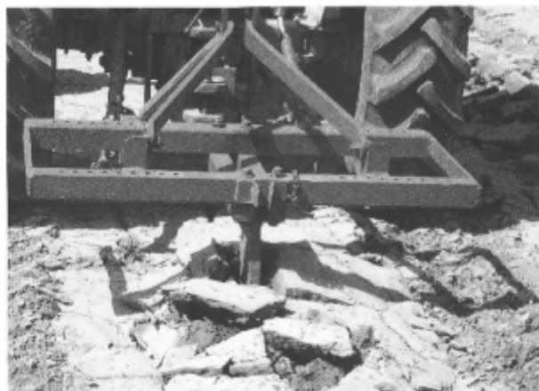
Figure 2: Sub soiling with tractor drawn chiseler
