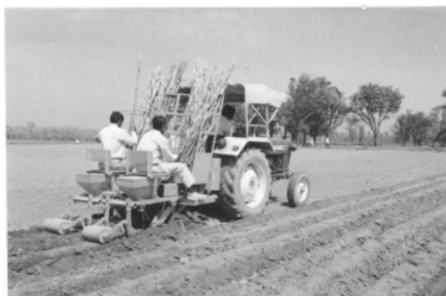
Figure 3: Two-row tractor operated sugarcane cutter planter
